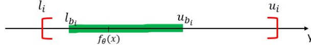
Figure 9: The general schematic of i^{th} output variable when upper and lower bounds of the variable are denoted by \mathbf{u}_i and \mathbf{l}_i and upper and lower bounds of the acceptable region are shown by \mathbf{u}_{b_i} and \mathbf{l}_{b_i} . The accepted region is shown in green colour.
