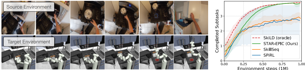
Figure 6: Semantic imitation from human demonstrations. Left: Qualitative state matching results. The top row displays frames subsampled from a task demonstration in the human kitchen source domain. The bottom row visualizes the states matched to the source frames via the procedure described in Section 4.3. The matched states represent corresponding semantic scenes in which the agent e.g., opens the microwave, turns on the stove or opens the cabinet. Right: Quantitative results on the kitchen manipulation task from human video demonstrations.
