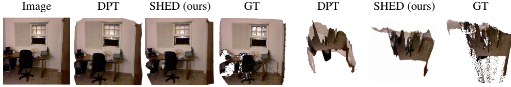
Figure 7: SHED produces structured 3D reconstructions. We visualize 3D point clouds reconstructed from single-view depth maps, following the semantic scene completion protocol (Song et al., 2017), using predictions from DPT, SHED, and the ground truth on NYUv2 examples. Frontal views (cols 2-4) show that DPT fails to preserve planar structures, producing curved wall boundaries, whereas SHED more accurately recovers straight lines. This difference is more apparent in the bird’s-eye views (cols 5-7): DPT yields warped surfaces, while SHED produces flatter layouts.
