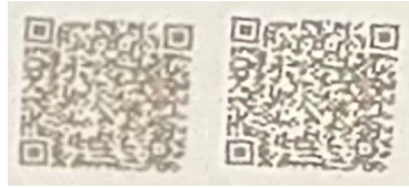
Figure 3: Super resolution input (left: not decodable) and output (right: decodable).
