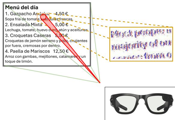
Figure 1. We use an event camera integrated on the Meta Aria glasses to perform object character recognition (OCR). Our event-based algorithm uses only the foveated events to perform binary image reconstruction and, then, OCR via large language models.
