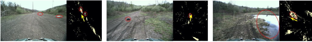
Figure 4: Example scenarios with geometrically-indistinct objects (tarps, tire, puddle) obstructing the path in red (robot pose is yellow arrow). The uncertainty layer classifies them as OOD objects.
