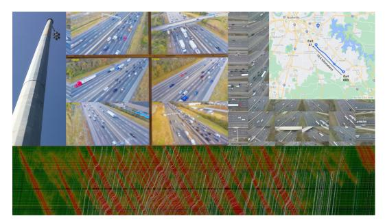
Figure 9: **I-24 MOTION illustration.** High-definition camera poles are mounted along a portion of I-24 at regular intervals. This generates massive amounts of video data, which is processed through a software stack. The resulting data for a single day is shown in the time-space diagram, displaying thousands of individual vehicle trajectories color-coded by speed (red for low speeds, green for high speeds), illustrating the complexity of the dataset.
