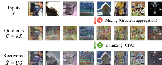
Figure 1. (a) Aggregate gradients from an FC layer are linear combinations of its inputs, as shown by the visualization of the gradients in the second row. (b) Cocktail party attack uses this observation to frame gradient inversion as a blind source separation problem and recovers the inputs from the gradients by optimizing an unmixing matrix U using independent component analysis.
