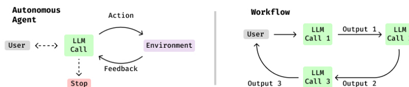
Figure 5: Agent architectures. Autonomous agents delegate branching decisions to the LLM, which chooses actions dynamically, while workflows follow a fixed, pre-defined sequence of calls.
