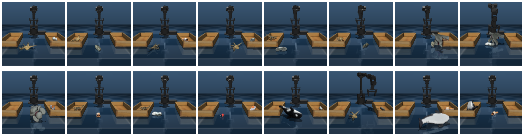
Figure 4: Observations from the Multi-Stage Manipulation environments consist of a single 128 \times 128 RGB image from a side camera and robot proprioception. The environment includes several different types of shoes and toys, which require different grasps. Moreover, their locations are randomized across the scene. Textures, lighting conditions, and camera angles are also varied across episodes.
