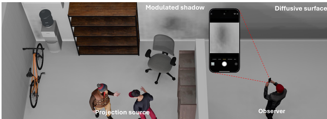
Figure 1: Scenario diagram. Projection source encodes gesture semantics into a spatiotemporally Modulated shadow projected onto a passive Diffusive surface . Observer recovers the original semantic information by observing the Modulated shadow .
