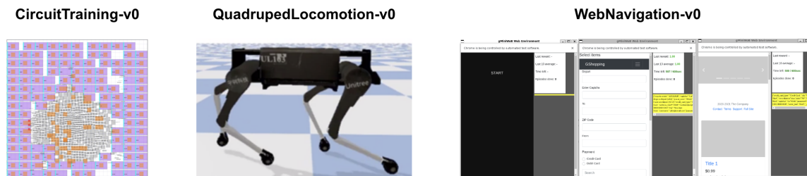
Figure 1: The three domains included in A2Perf: computer chip floorplanning for optimizing integrated circuit layouts, web navigation for automated form filling and website interaction, and quadruped locomotion for robotic control. These specific domains were selected based on their demonstrated transfer from simulation to real-world applications.
