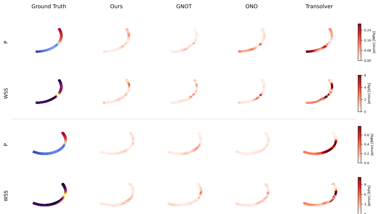
Figure 8: Pointwise absolute prediction error on two single-vessel test geometries, following the same layout as Figure 3. Our model (128 RBFs) attains relative \ell_2 errors of 3.51%/5.83% and 2.74%/5.18% (P/WSS). GNOT (3.15%/5.95%, 3.87%/5.83%) and ONO (5.29%/8.16%, 2.32%/5.11%) are competitive on single-vessel data, while Transolver shows higher error (11.54%/20.85%, 17.19%/21.65%).
