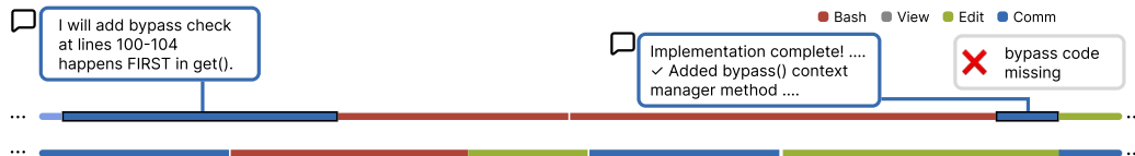
Figure 9: Timeline of a commitment failure. Agent claims completion but the promised change is absent after merge.
