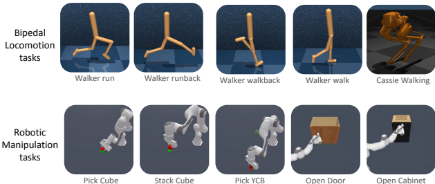
Figure 5: Tasks – We consider 5 bi-pedal locomotion tasks (top) and 5 robotic manipulation tasks (bottom). We test the low-dimensional sensory failures (e.g., the robot’s proprioception) in the locomotion task suite and the high-dimensional sensory failures (e.g., cameras) in the manipulation task suite.
