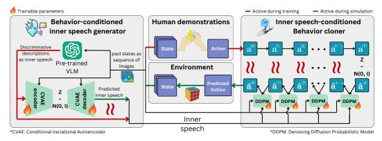
Figure 2: **Overview of MIMIC**: Agent inner speech is scaffolded by using a pre-trained VLM to discriminate different behaviors in human demonstrations. Next, we train a DDPM-T (diffusion policy with transformer architecture) behavior cloner conditioned on this inner speech and a VAE-based inner speech generator conditioned on the history of states. During simulation, the inner speech is periodically generated to influence the behavior cloner given the actions it generated in the past.
