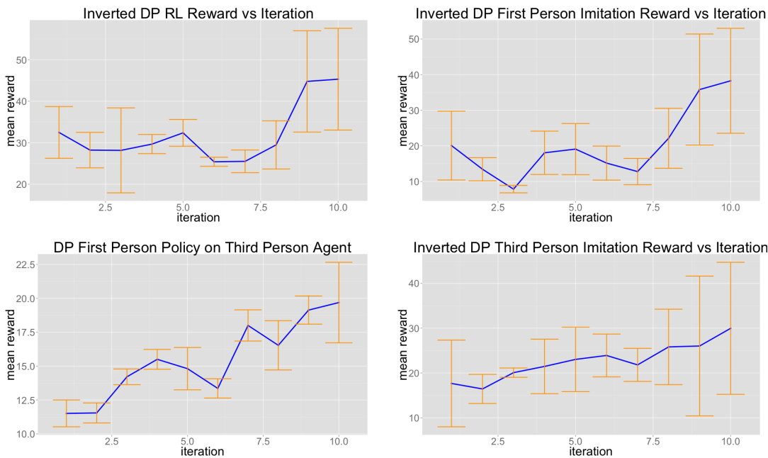
Figure 10: Inverted Pendulum performance under a policy trained on RL, first-person imitation learning, third-person imitation, and a first-person policy applied to a third-person agent.
