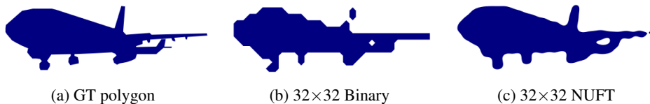
Figure 8: Visualizing different representations. (a) Shows the original ground truth polygon, (b, c) show reconstructed polygons from binary and NUFT representations.
