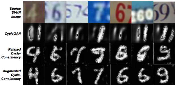
Figure 5: Qualitative comparison of domain adaptation for experimental models. Each column illustrates the mapping performed by each of the models from the original SVHN image (source domain) to MNIST (target domain, 10 labeled samples per class in total). It can be seen that the augmented cycle-consistent model is able to preserve most of the semantic information, while still approximately match the target distribution.
