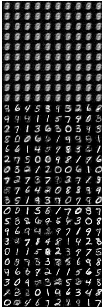
Figure 7: All 100 Prototypes learned using linear ( top ), dense ( middle ), and CNN discriminator ( bottom ). We observe that with linear discriminator, only the mean of the training set is learned, while using the dense discriminator yields blurry prototypes. Only the CNN discriminator yields clear prototypes.
