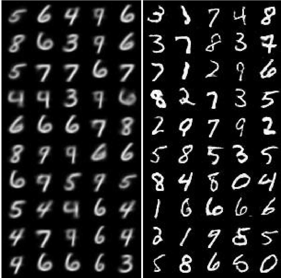
Figure 11: VAE ( left ) and GAN ( right ) samples with 200 latent variables. Each row represents a sample of a combination of 5 digits generated by the model.
