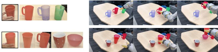
Figure 7: Robot experiment of grasping the object that is closest to the query object (held by hand). Images on the left are captured by the robot camera, and the images on the right are the video frames from a third person view camera. The leftmost object (black border) is the query object and its nearest neighbors are listed in descending order. The top row and the bottom row show the robot successfully identifies and grasps the object with similar color and shape attribute respectively.
