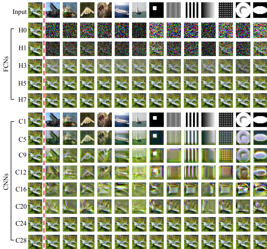
Figure 43: Visualization of predictions from various networks trained on a single CIFAR-10 image (air plane). The first row shows the input images, where the first one is the training image and the rest are images for evaluation. The evaluation images consist of unseen images from the CIFAR-10 test set and artificially generated grayscale patterns. The grayscale patterns are duplicated into three channels before feeding into the networks. The remaining rows show the predictions from trained FCNs and CNNs. For FCNs, the numbers indicate the number of hidden layers. For example, H3 means a 3-hidden-layer FCN. For CNNs, the numbers indicate the number of (convolutional) layers. For example, C16 means a 16-layer CNN.
