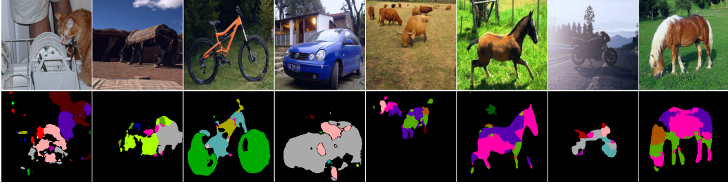
Figure 4: Illustration of the checkerboard problem in semantic segmentation using deconvolutional layers. The first and second rows are the original images and semantic segmentation results, respectively.
