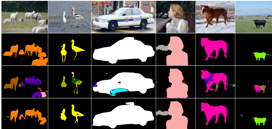
Figure 1: Comparison of semantic segmentation results. The first and second rows are images and ground true labels, respectively. The third and fourth rows are the results of using regular deconvolution and our proposed pixel deconvolution PixelDCL, respectively.
