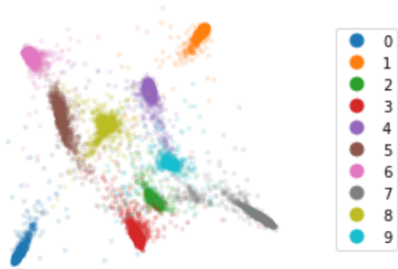
Figure 7: Linear projection of the embedding obtained by applying the MIB encoder to the MNIST test set. The 64 dimensional representation is projected onto the two principal components. Different colors are used to represent the 10 digit classes.
