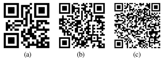
Fig. 2. (a) Version 1 QR code with 21 \times 21 square dots; (b) Version 3 QR code with 29 \times 29 square dots; (c) Version 5 QR code with 37 \times 37 square dots.
