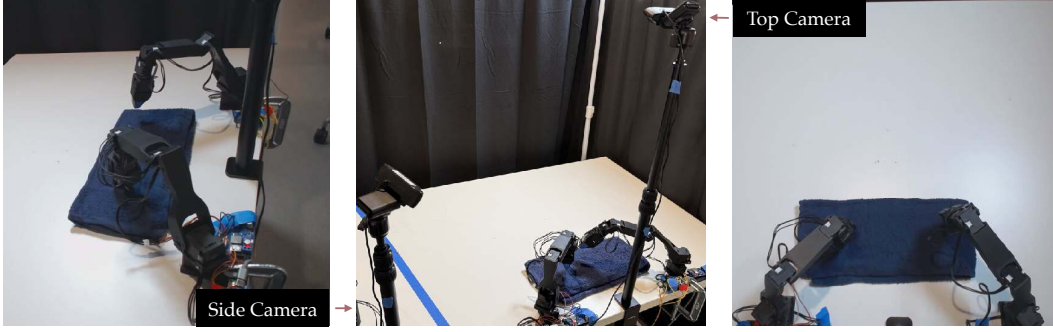
Figure 10: Real World Bimanual Robot Setup. Our real-world setup consists of a top-down and side camera mounted to a table where two Koch v1.1 low-cost arms are mounted. This setup allows us to perform bimanual tasks and easily collect data with another pair of low-cost “leader” arms mounted to the same table.
