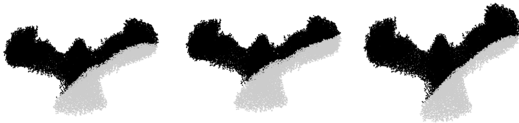
Figure 20: Ablation study on the material and size. Black points represent solid part and grey points represent hollow part. The first graph is the original setting. The second graph is doubling the scale of the hawk. The third graph is doubling the material density of the hawk. We can observe that with the same relative shape and relative physical parameters, the output does not change with its absolute value.
