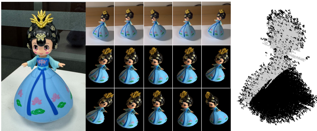
Figure 6: Wobbly doll (Sec. 8.3). Left: a photo of the wobbly doll. Middle: frames from a video recording of the harmonic oscillation of the doll (top), simulated motion with an interior design optimized from our pipeline (middle), simulated motion of a solid doll (bottom). Right: a cross-section visualization of the optimized interior geometry from our pipeline, where black represents solid part and grey represents hollow part.
