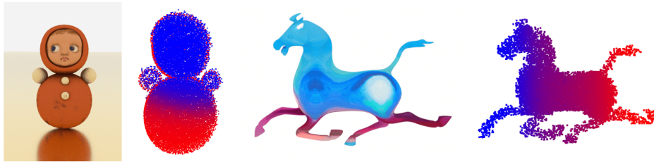
Figure 23: Experiments which supports continuously varying material. The two experiments share similar setting with the previous wobble doll and horse experiment, while the main difference is we allow a continuously varying material. The first and third figures are two typical input images, while the second and fourth figures are the optimized result. The color indicates the density of each point, where red means higher density (solid) and blue means lower density (hollow).
