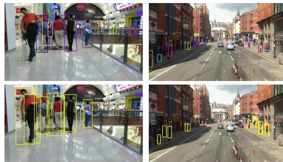
Figure 1: Discrepancy between GT bounding box (top) and the public detections provided by MOT benchmark datasets (bottom): the GT contains boxes for an occluded target, and the detection box is missing or includes false positives in the on provided detections.
