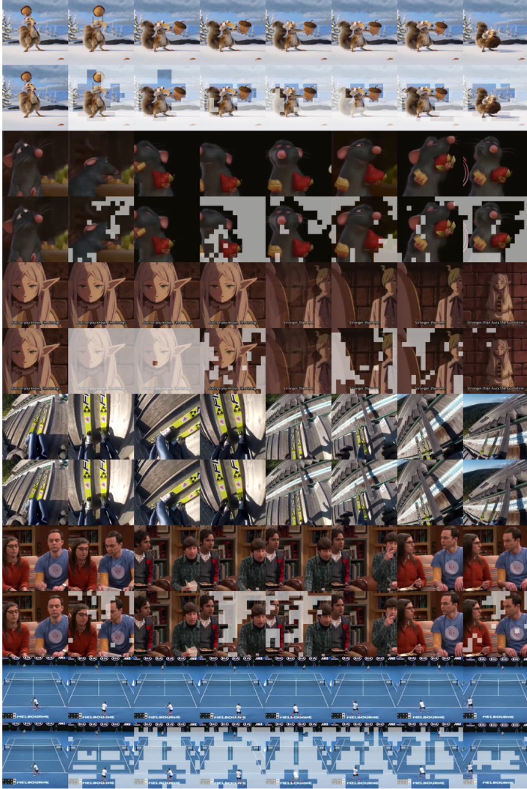
Figure 5: More examples. We visualize RLT’s effect on videos ranging from TV shows, movies, action sequences on a GoPro, and sports. RLT consistently prunes out tokens that are repeated and static, and includes all patches that change between frames, retaining as much information as possible while cutting the number of tokens significantly.
