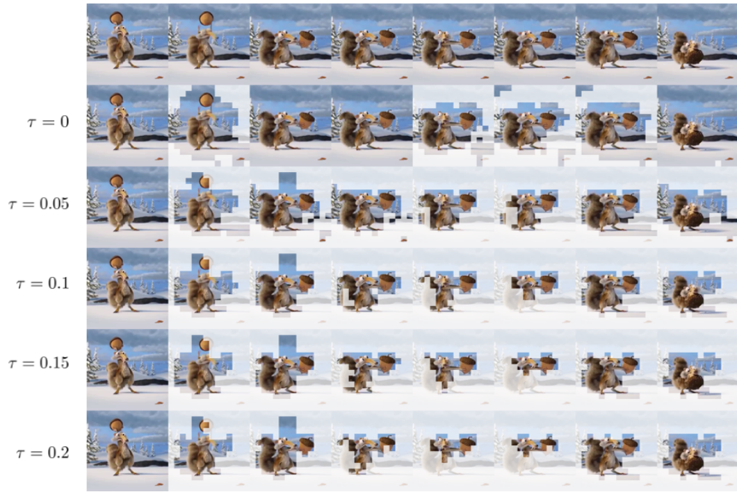
Figure 6: Effect of \tau . With low values of \tau , the clearest repeated patches are ablated, but imperceptible variations can prevent some visibly similar tokens from being pruned. Above \tau = 0.1 , some tokens with slight movement are pruned.
