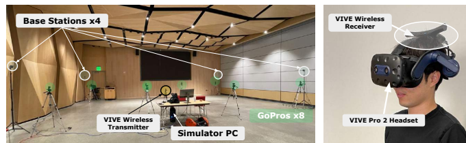
Fig. 3: Left: The VR system set up in the classroom data collection space. Right: A pedestrian subject wearing the VR headset.
