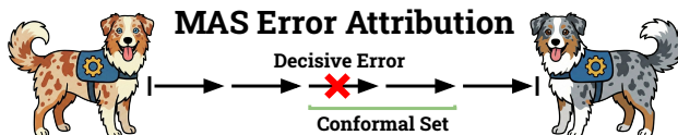
Figure 1. Conformal agent error attribution isolates the decisive error in a failed MAS trajectory within a conformal prediction set, providing statistical guarantees of coverage.
