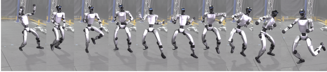
(a) Dynamic motion tracking: The FPO++ policy reliably tracks long (1.5-minute) and highly dynamic dancing motions from the LAFAN dataset entirely onboard.
