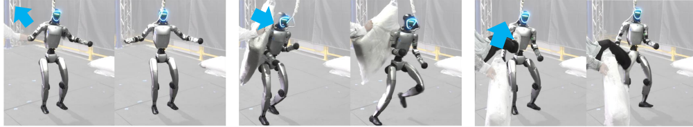
(b) Robustness to Perturbations: The FPO++ policy exhibits strong robustness against external forces and pushes, maintaining balance and continuing to track the reference motion despite significant disturbances.
