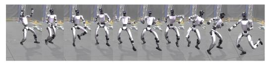
(a) **FPO++ motion tracking with a Unitree G1 robot.** We train BeyondMimic (Liao et al., 2025)-style motion tracking using a flow matching policy, which is deployed directly to the G1 robot.
