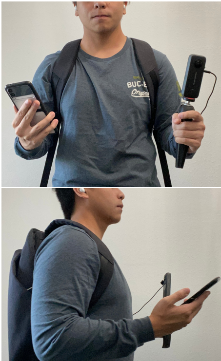
Figure 2: Viewer-Centric design: 360-degree camera, adjustable backpack, two (2) mobile devices (one in hand and one in backpack), and a battery bank inside backpack
