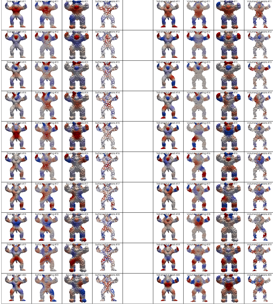
Figure 11: Eigenvectors 11 to 20 on the Armadillo, understood as a surface on the left and as a volume on the right. From left to right, the shape is encoded as a triangle mesh, a point cloud sampled uniformly at random, a voxel grid, a Gaussian mixture; a tetrahedral mesh, a point cloud, a binary mask and a Gaussian mixture.
