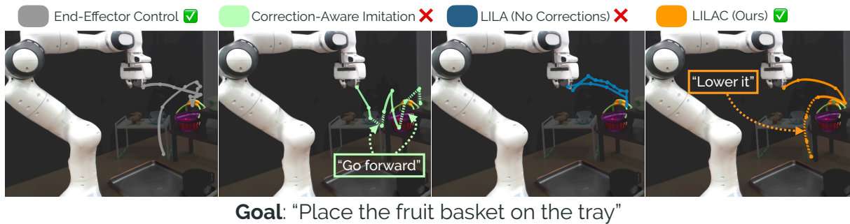
Figure 3: Qualitative trajectories from 4 different control strategies, operated by an “oracle.” Note the dashed lines indicate when language corrections were used. In general, both LILAC and the End-Effector control methods are able to solve tasks, with LILAC able to do so more efficiently. Imitation Learning (green) fails to fit the tasks – even with corrections – and LILA is unable to progress without finer-grained correction information.
