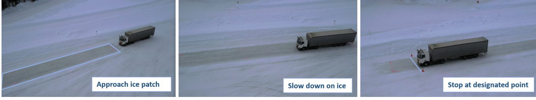
Figure 4: As the truck approaches a previously unobserved ice patch on a slippery road, MetaKoopman enables the planner to adapt, allowing the vehicle to brake accurately on a low friction surface.
