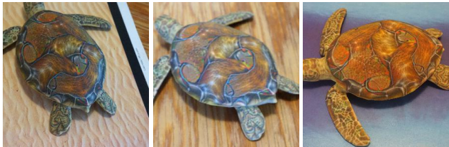
Figure 6: Three pictures of the same adversarial turtle (all classified as “rifle”), demonstrating the need for a wide distribution, and the efficacy of EOT in finding examples robust across wide distributions of physical-world effects like lighting.
