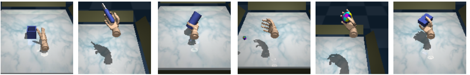
Figure 1: Figure showing some of the objects and their grasps by the model (snapshot at different time intervals). Left to right, a can, screw driver, cylinder, coin, ellipsoid and cuboid are shown. The table is bounded by four walls (green in color) that can be seen
