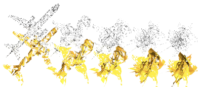
Figure 3: Meshing a point cloud and then applying Laplacian smoothing as in (Taubin, 1995). Corresponding point clouds attached above.
