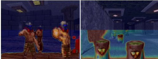
Figure 10: Examples of affordance maps \hat{y} predicted by the navigability module, showing accurate localization of semantic constraints within the scene. (Left) contains dynamic hazards in the form of monsters and (Right) contains areas of geometry-affordance mismatch, in the form of barrels shorter than sensor height.
