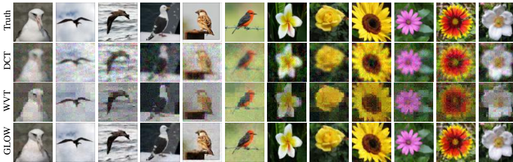
Figure 38: Compressed sensing — Visual comparisons on the test set images from Birds and Flowers dataset with a number m = 2,500 ( \approx 20\% ) of measurements under the Glow prior, LASSO-WVT, and LASSO-DCT at a noise level \sqrt{\mathbb{E}\|\eta\|^2} = 0.1 . In each case, we choose values of the penalization parameter \gamma to yield the best performance among the tested values. We use \gamma = 0 for Glow prior and \gamma = 0.01 for LASSO-WVT, and LASSO-DCT, respectively.
