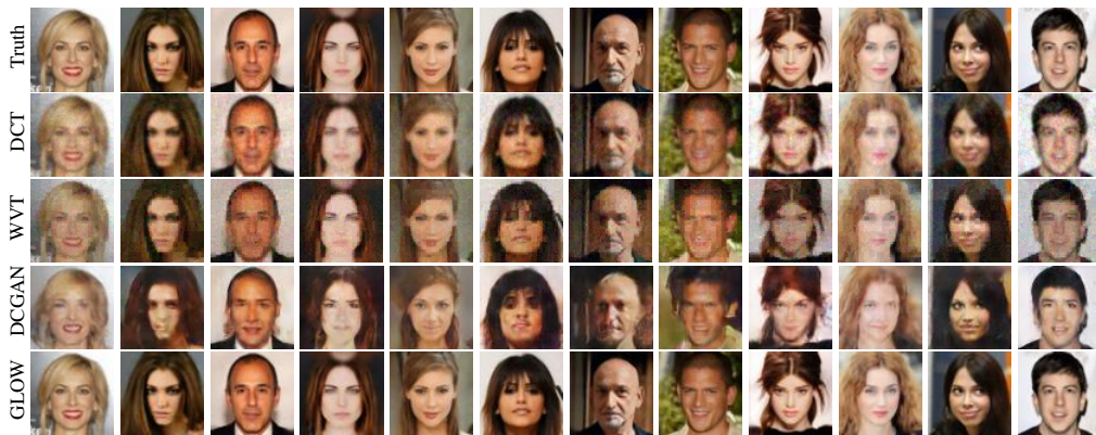
Figure 28: Compressed sensing visual comparisons — Recoveries on (within-distribution) test set images with a number m = 5000 ( \approx 41\% ) of measurements under the Glow prior, the DCGAN prior, LASSO-WVT, and LASSO-DCT at a noise level \sqrt{\mathbb{E}\|\eta\|^2} = 0.1 . In each case, we choose values of the penalization parameter \gamma to yield the best performance among the tested values. We use \gamma = 0 for both DCGAN, and Glow prior and \gamma = 0.01 for LASSO-WVT, and LASSO-DCT, respectively.
