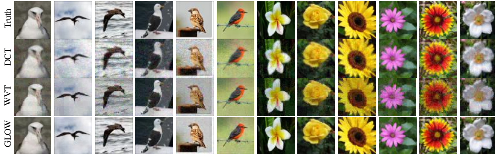
Figure 39: Compressed sensing — Visual comparisons on the test set images from Birds and Flowers dataset with a number m = 5,000 ( \approx 41\% ) of measurements under the Glow prior, LASSO-WVT, and LASSO-DCT at a noise level \sqrt{\mathbb{E}\|\eta\|^2} = 0.1 . In each case, we choose values of the penalization parameter \gamma to yield the best performance among the tested values. We use \gamma = 0 for Glow prior and \gamma = 0.01 for LASSO-WVT, and LASSO-DCT, respectively.
