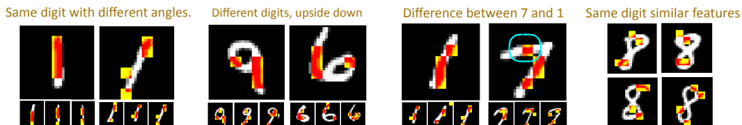
Figure 3: The hand-written digits and explanations provided by VIBI were randomly selected from the validation set. The selected patches are colored red if the pixel is activated (i.e. white) and yellow otherwise (i.e. black). A patch composed of 4 \times 4 pixels is used as a cognitive chunk and k = 4 patches are identified for each image.
