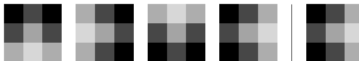
Figure 1: Left: image patches with various orientations. Within convolutional neural networks, these patches would have to be detected with respectively equally oriented filters. Right: Images after centroid rotation. With rotational invariance, all four patches would be mapped to the same orientation.
