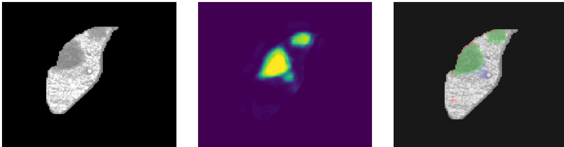
Figure 3: Exemplary segmentation result using rotationally invariant filters. Left: original image; middle: segmentation result; right: overlay. True positives, false positives and false negatives are respectively marked as green, blue, and red.
