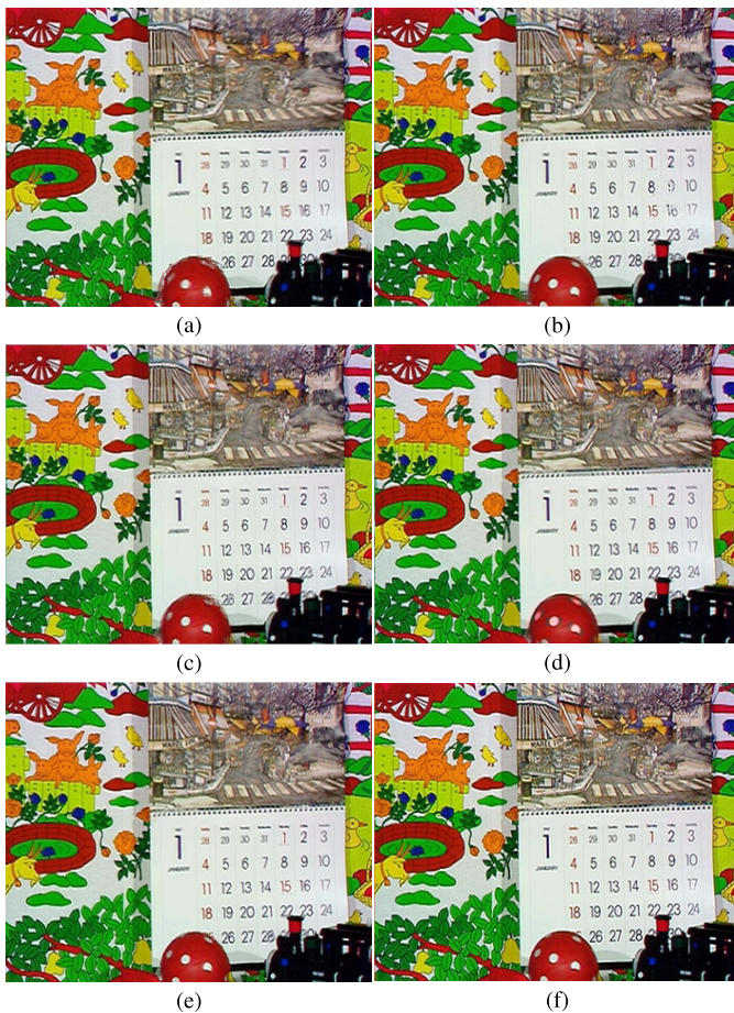
Fig. 4. Subjective comparison of Mobile 's 12-th frame. (a) Kim and Sunwoo [28], 24.88dB. (b) Kaviani and Shirani [24], 28.31dB. (c) Lee et al. [23], 27.87dB. (d) Guo et al. [27], 27.22dB. (e) HOMDF, 28.74dB. (f) Groundtruth.
