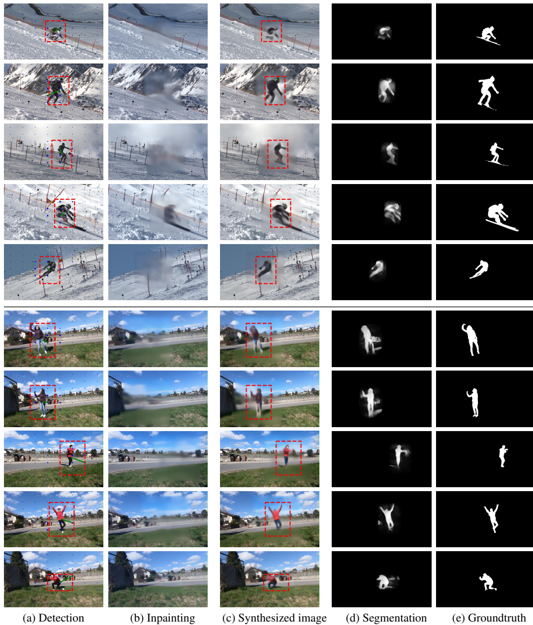
Figure 9: Detection and segmentation results on the test subjects of Ski-PTZ-camera and Hand-held190k dataset. (a) Detection result. The blue dots coincide with the grid cell centers and their size indicates the confidence of the bounding box proposals. The selected bounding box is illustrated with a red dashed line and the center of the grid cell yielding this proposal is connected to the center of the red box through the green line. (b) The inpainting result where the region inside the detected bounding box is reconstructed by our inpainting network (only needed for training). (c) The synthesized image with the predicted foreground and background regions combined. (d) Segmentation mask result. (e) Groundtruth segmentation mask.
