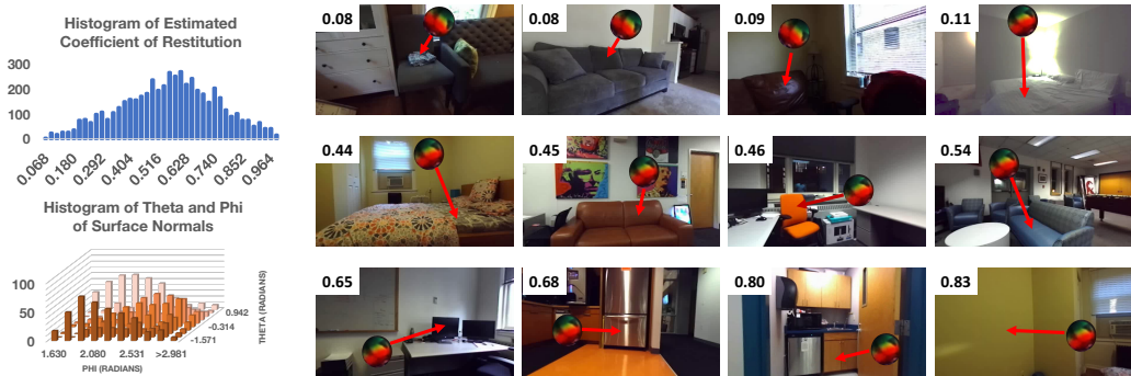
Figure 5: Our collected Bounce Dataset of 5K real-world bounces. Our dataset spans a variety of real-world everyday scenes. In each image we mark the location of the observed bounce and show the estimated coefficient of restitution at the top-left. Larger values correspond to harder surfaces such as floors and countertops.
