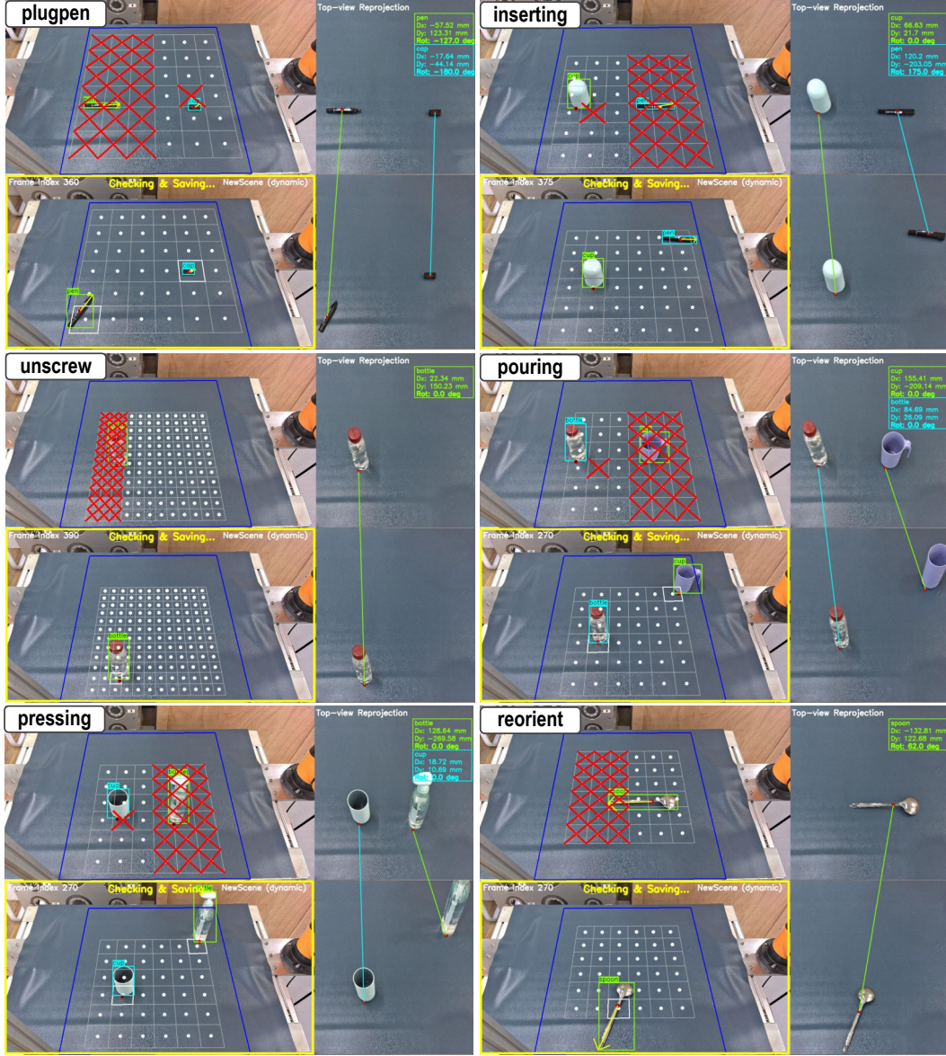
Figure 11: UI interface examples. When collecting data, the six tasks need to display different grid cells in real time, as well as perceive and track objects related to the tasks. Note that these points, crosses and lines are drawn digitally, which are not marks in the real world.
