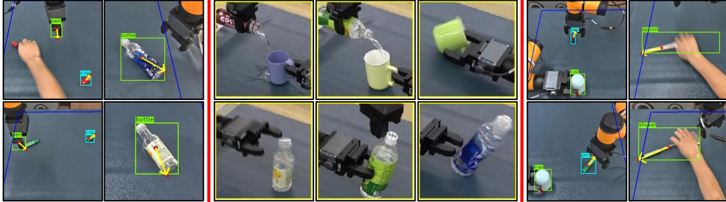
Figure 14: Typical failure cases. Left four cases: These include two cases from the plugpen task that incorrectly detected the marker body, and two cases from the reorient+unscrew task that incorrectly estimated the lying bottle’s orientation. Middle six cases: These include three cases from the pouring task where water was spilled or the mug cup was misgrabbed, and three cases from the unscrew task where the gripper failed to grab the bottle’s body or cap accurately (these are extra footages from a third-person perspective). Right four cases: These include two cases in the inserting task where the robotic arm’s end effector occasionally obscures the marker pen, and two cases in the reorient task where human interference causes the hand to partially obscure the spoon/shovel. Here, visual perceptual defects do not necessarily lead to task failure, demonstrating the robustness of the proposed orientation estimation algorithm.
