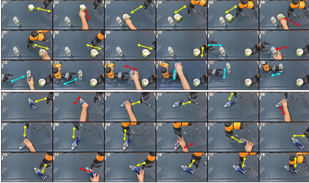
Figure 16: Qualitative examples of applying dynamic interferences during the pre-grasping execution. From top to bottom, they are segments of the dynamic closed-loop grasping phase of tasks pouring and reorient+unscrew, where each object is manually disturbed from one to three times. The red arrow indicates the direction of the manually moved object (interfering). The cyan arrow and yellow arrow indicate the movement direction of the left and right robotic arms (chasing) respectively. Best to view after zooming in.
