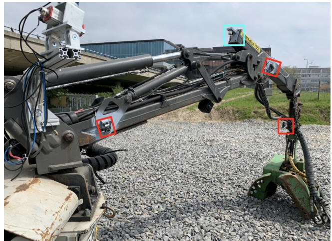
Fig. 4. Mounting location of proprioceptive sensors. Inertial sensors are shown in red and the encoder in turquoise color. Note that the IMU sensors are mounted as close as possible to the joint axis to minimize the inertial forces measured by the sensor.
