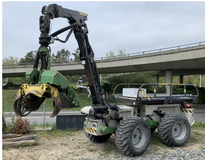
Fig. 1. Harveri harvester parked on our testing field. Automating the machine is currently a work in progress.
