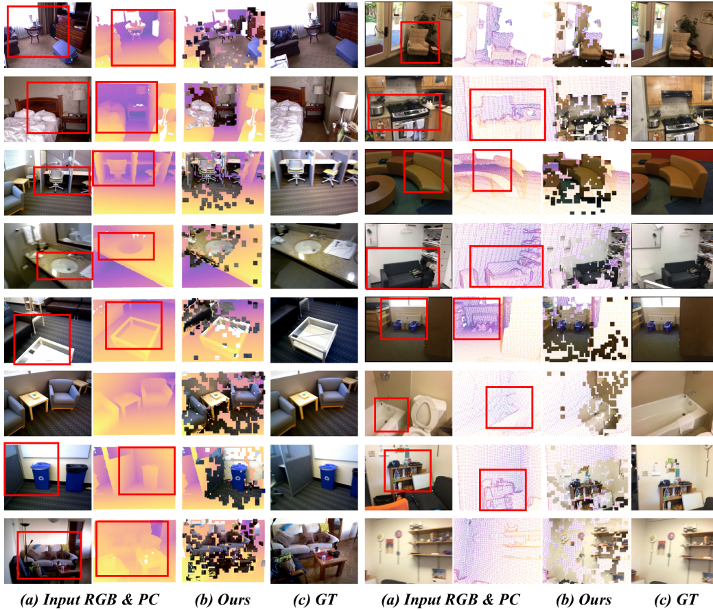
Figure 10: Patch warping results. Based on the estimated FreeReg correspondences, we warp the 32 \times 32 local RGB patches to their estimated corresponding positions in the point cloud. (a)The input RGB and depth images. (b)The RGB patch warping results are based on the established correspondences of FreeReg. (c) The ground truth RGB image of the input depth map.
