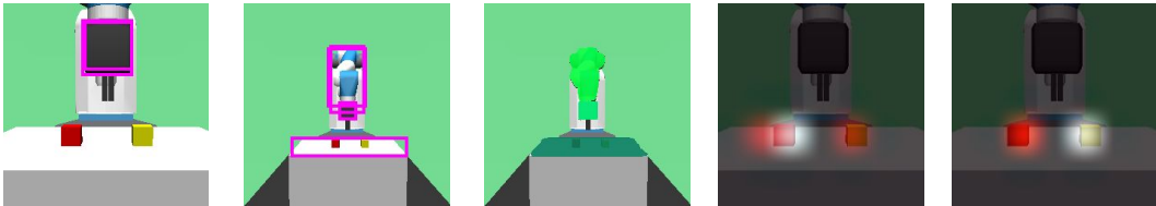
Figure 3: a) Mask R-CNN object detection results b) Mask R-CNN detection results on far view c) Mask R-CNN instance segmentation results on far view d) Grad-CAM result with 'red block' text input (white being highest intensity) e) Grad-CAM result with 'yellow block' text input (white being highest intensity).
